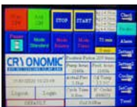
Touchscreen control panel
