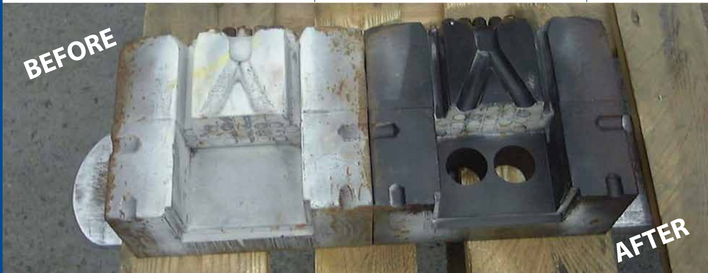
Mould cleaning in foundries : result after 2 minutes of dry ice blasting!
